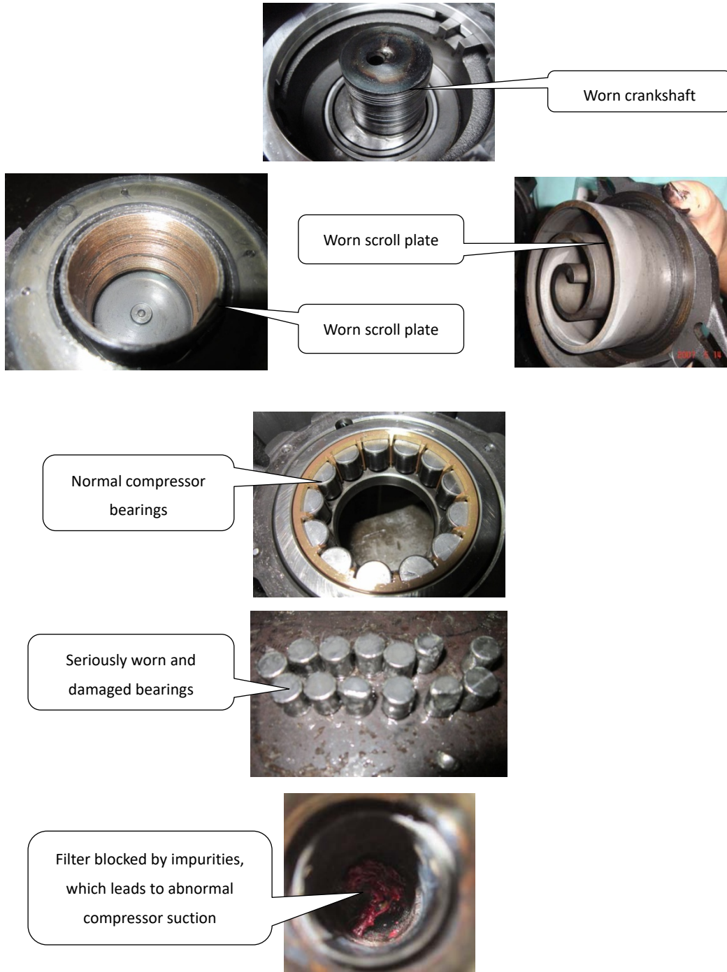
Figure 6-2.11: Effects of spoiled compressor oil
