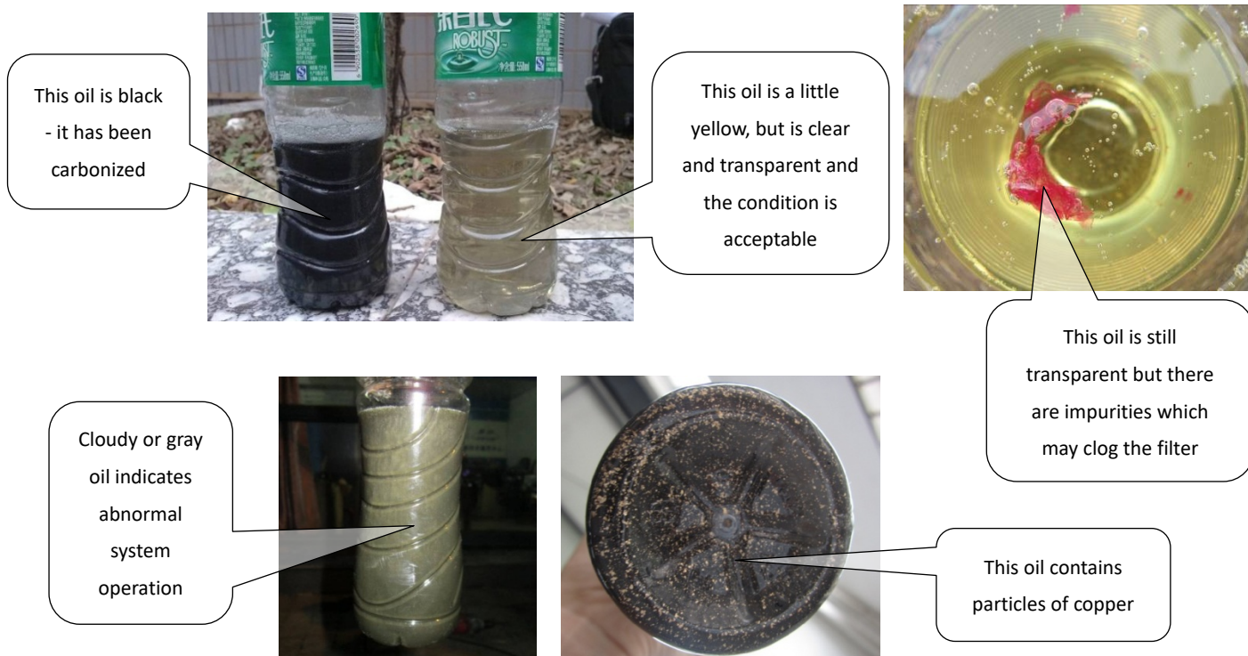
Figure 6-2.10: Inspecting compressor oil
