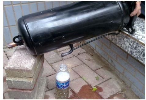
Figure 6-2.8: Draining oil from a compressor
