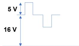
F1-F2 terminals on indoor units, branch selector boxes, outdoor units and central controllers are all possible measurement points. Use as many points as you can and take the time necessary for measurement if analyzing with an oscilloscope.
