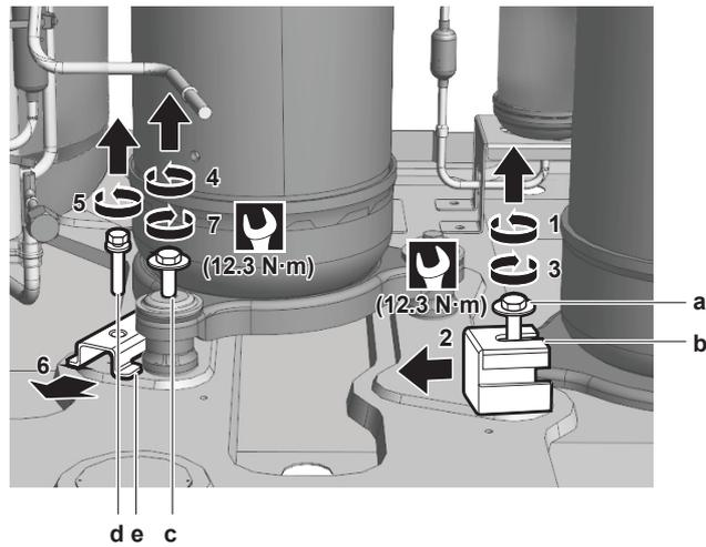
**To remove the compressor insulation**
