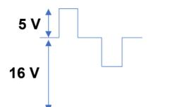
F1-F2 terminals on indoor units, BP-units, outdoor units and central controllers are all possible measurement points. Use as many points as you can and take the time necessary for measurement if analyzing with an oscilloscope.
