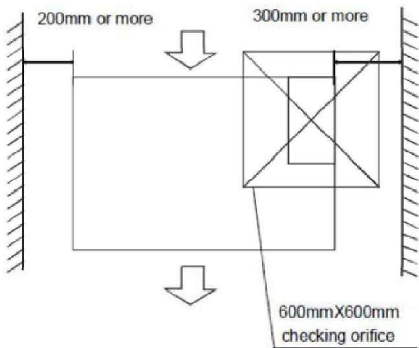
There is enough space for installation and maintenance. The ceiling is horizontal, and its structure can endure the weight of the indoor unit. The outlet and the inlet are not impeded, and the influence of external air is the least. The air flow can reach throughout the room. The connecting pipe and drainpipe could be extracted out easily. There is no direct radiation from heater.
