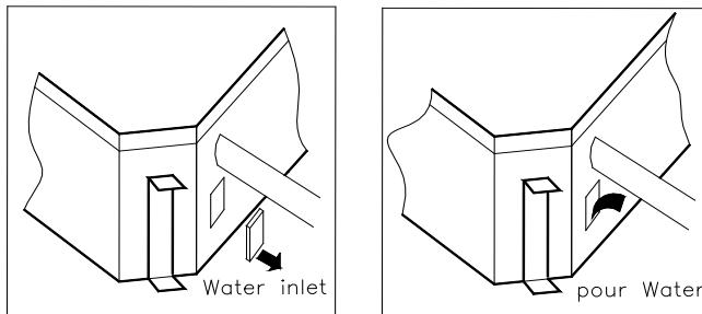
② Turn on the power to Cooling operation. Check the pump's operation and switch on the Water Level Switch. Check the pump's sound and look into the transparent hard pipe in the outlet at the same time to check if the water can discharge normally.
