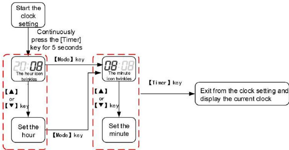
Set the period by pressing the [Timer] key and then exit from the clock setting with such setting saved;
