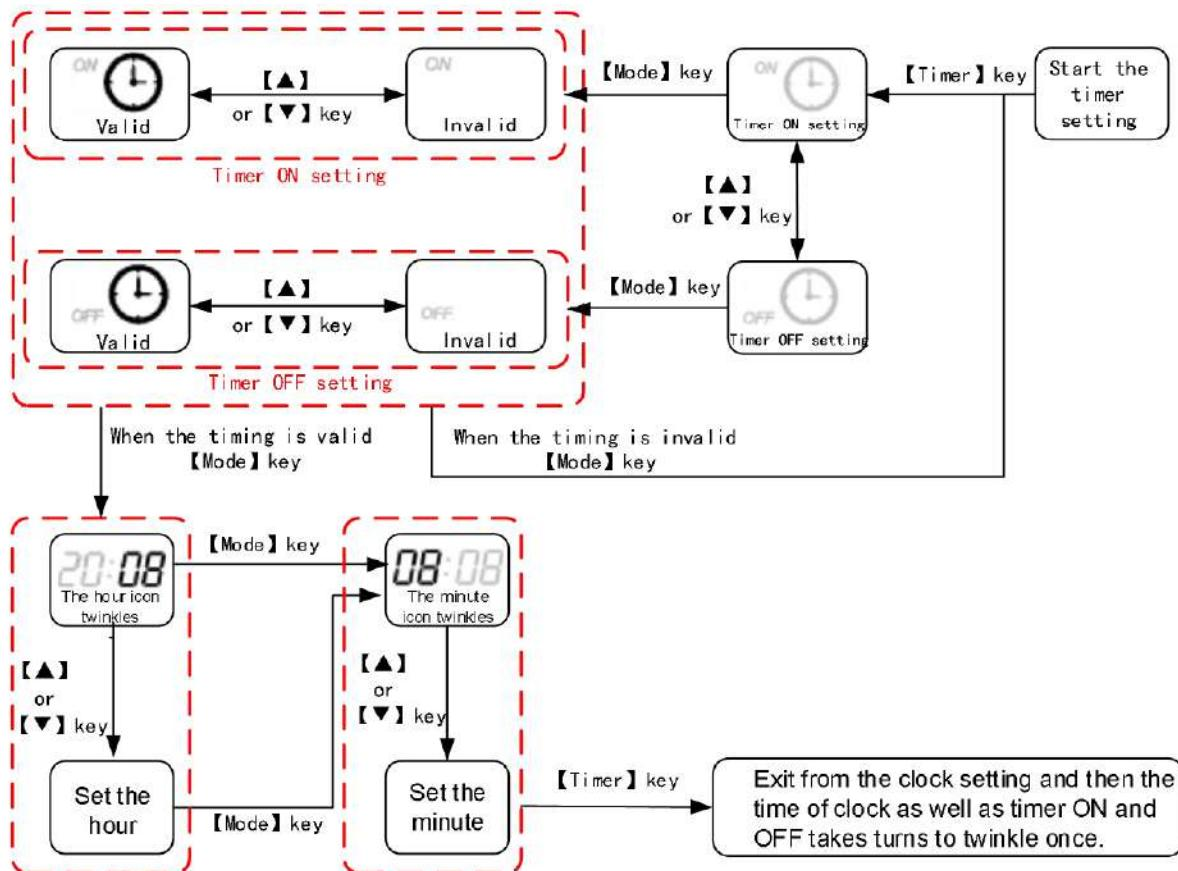
Set the period by pressing the [Timer] key and then exit from the clock setting with such setting saved;
